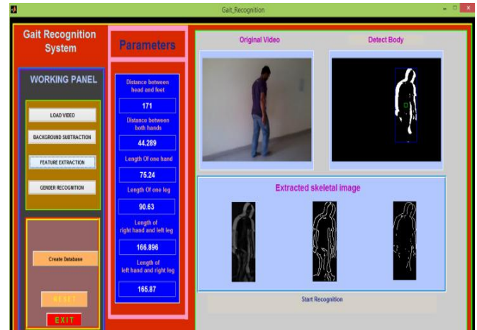
Fig 2: Feature Extraction and parameters involved in recognizing various Walking directions of a human.
