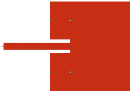
Figure 1: Layout of 1x1 Patch Antenna with Inset Feed
