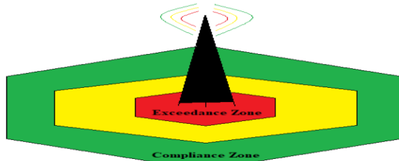
Figure 2: EMF exposure zones around a base station antenna
